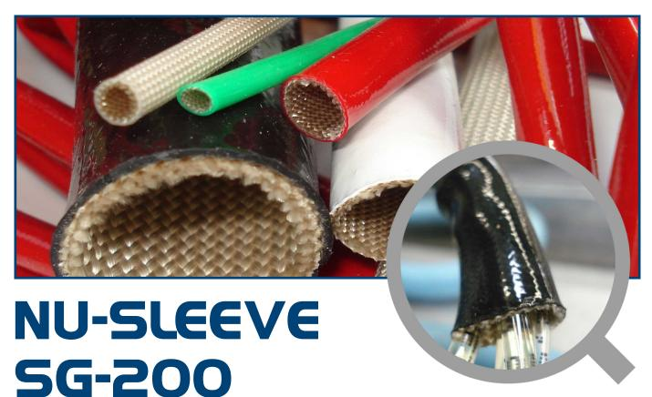
NU-SLEEVE SG-200 is available in 5 electrical grades (A, B, C-1, C-2 and C-3) in a standard wall (NEMA TF-1, Table 3-1) construction. All grades are made using braided E-Glass yarns that have been heat treated to optimize coating adhesion and minimize surface irregularities and then coated with liquid silicone rubber (LSR). LSR products are available in Grades A, B, C-1, C-2 and C-3.
